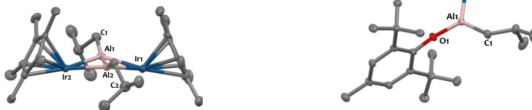
Figure 2. Solid-state structures of [\text{IrCp}^*\text{H}_2\text{Al}(\text{Bu})_2] (left) and [\text{IrCp}^*\text{H}_2\text{Al}(\text{Bu})(\text{OAr})] (right) complexes determined by single-crystal X-ray diffraction.
